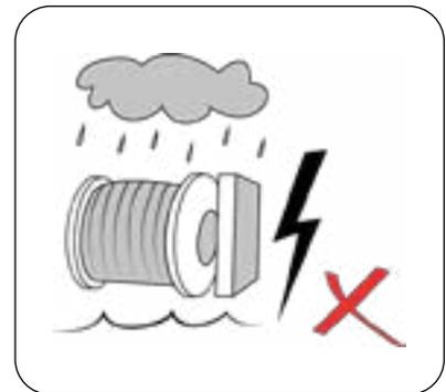
**6.** Do not use the hoist under the rain. Do not wet the engine or the switch.
