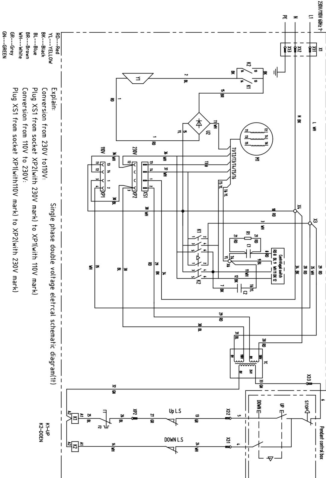
8.3. Trolley Wiring Diagram (All models)
